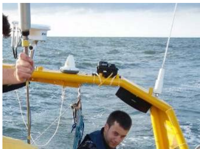
Photo left : INMARSAT transmitter beside the (black) Top-Box with PAR sensor and GPS receiver.
